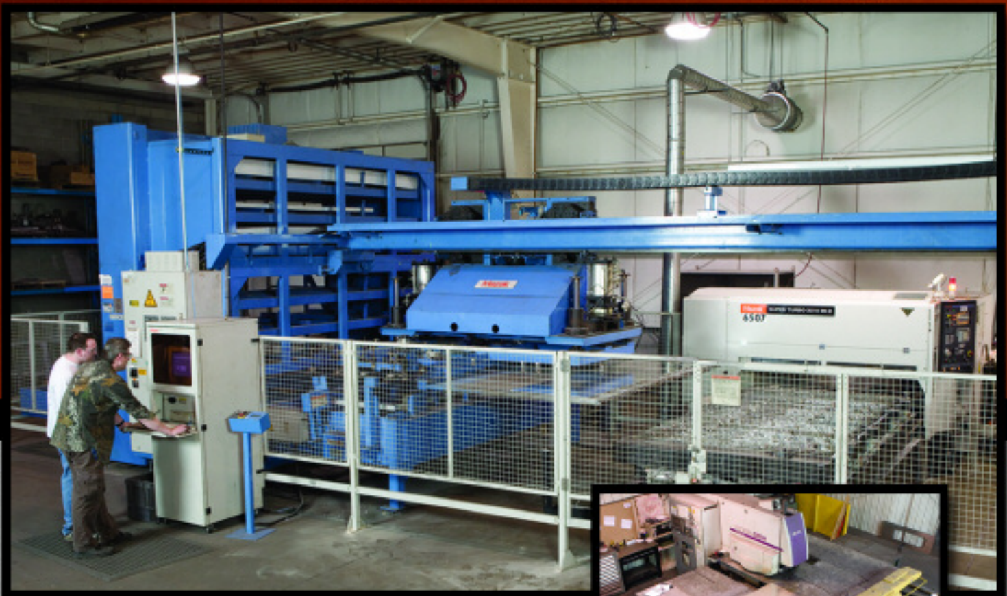
Our 4000 Watt, 5 x 10, Mark II laser is shown fully equipped with a Flexible Manufacturing System. FMS allows for material to be stored, retrieved, and pneumatically loaded, resulting in less set-up and down time and providing you with a lower total cost.
